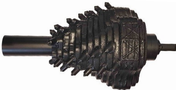
Fluted-Reamer with integrated Swivel made of plates
